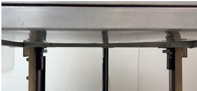
Film sag too shallow; may lead to poor corner heating.
