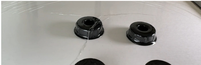
Wrinkling caused by excess surface area from overheating.
