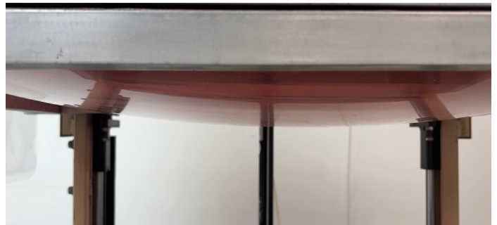
Proper sag benchmark: approximately 3–4 inches.
