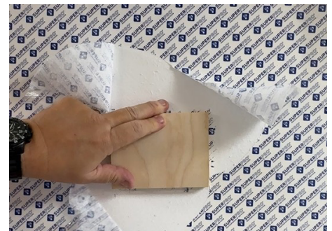
Peel test showing fiber tear, indicating a strong seal.
