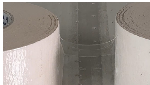
Film bridging between products due to spacing/height issues.
